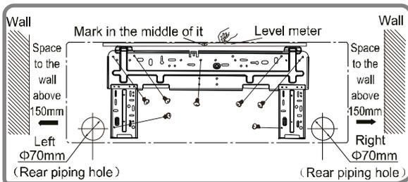
Drill a piping hole of diameter  $\Phi 55$  or  $70$  at the chosen location for the outlet pipe. To allow for proper drainage, the piping hole in the wall must slant slightly downwards to the outdoor side, with a gradient of  $5 - 10^\circ$ .
