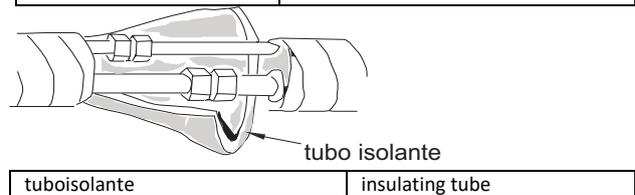
Wrap the indoor pipe and the joint of the connecting pipe with an insulating tube. Then wrap with tape.
