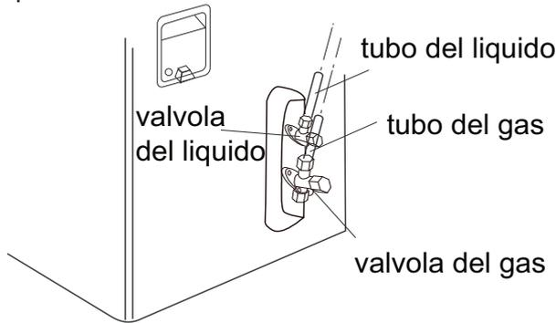
4. Tighten the union nut with the wrench according to the following table.
